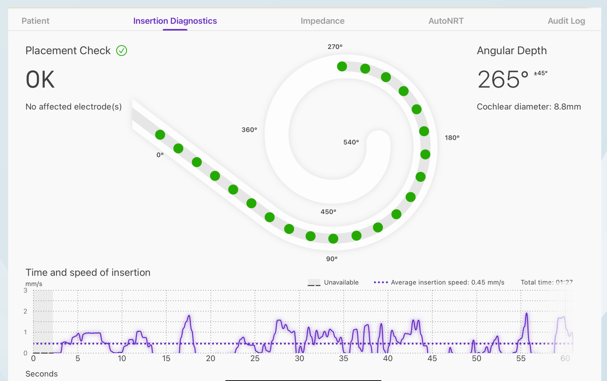
Fig 8 Initial display of SmartNav showing no tip foldover but low angular depth
