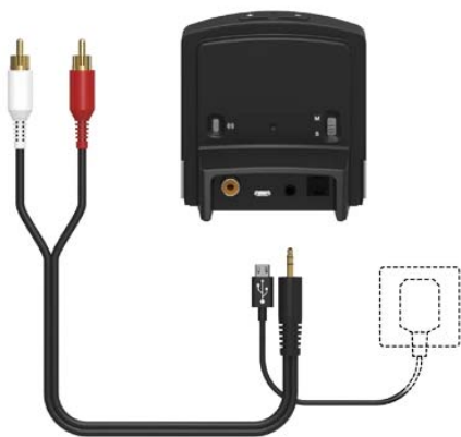
Typical connection to TV or stereo
