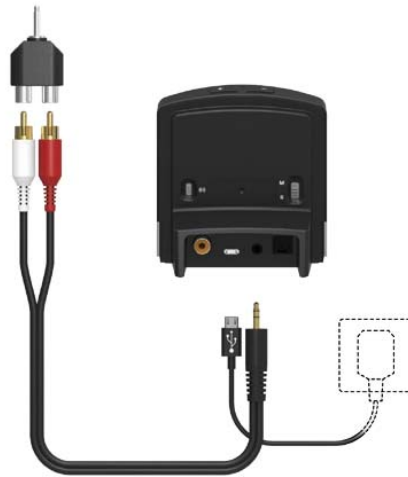
Typical connection to computer headphone terminal
