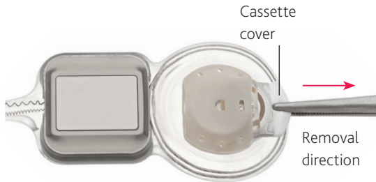
Figure 24: CI622 implant with cassette partially removed
