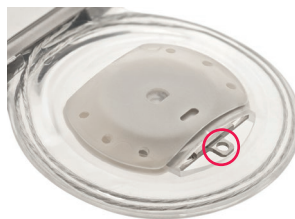
Figure 19: Metal tab on magnet cassette
