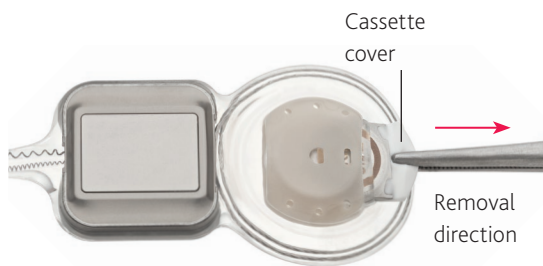
Figure 33: CI632 implant with cassette partially removed
